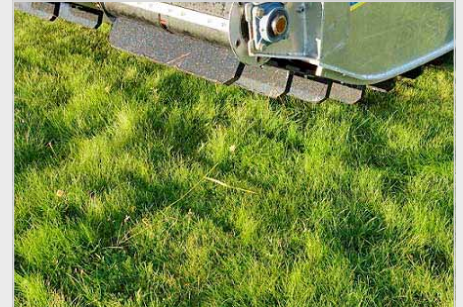
The Truxor's weight distribution system minimizes ground pressure. Truxor can be driven across a lawn without any damage to the grass.
