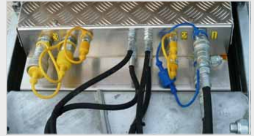
Hydraulic outlet for operation of tools. Operated by an on/off joystick as well as min/max tool speed.
