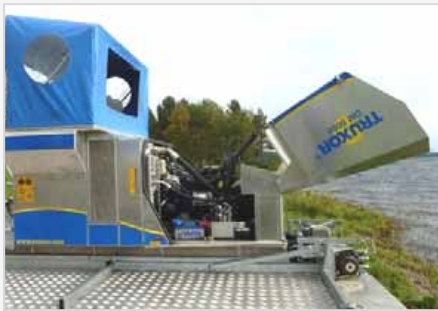
Openable engine casing with a tool box inside the engine compartment.
