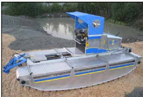
The movable driver's cab is hydraulically adjusted and works as counterweight during heavy lifts in water.
