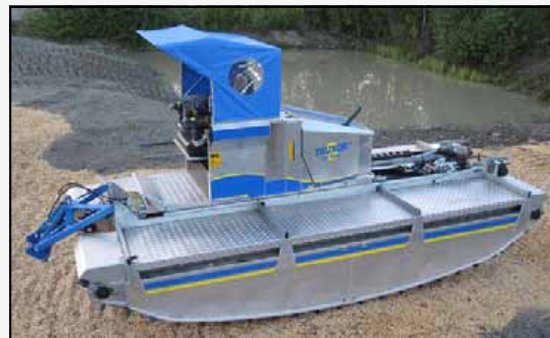
The movable driver's cab is hydraulically adjusted and works as counterweight during heavy lifts in water.
