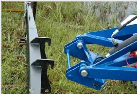
The DM bracket makes tool change easy.
