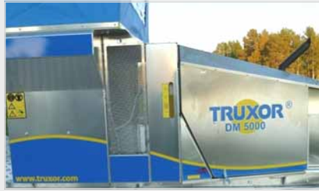
The air intake to the radiator is equipped with a filter that prevents the cooler cells from being blocked by insects and foreign particles.
