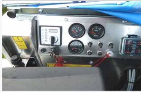
The dashboard shows hydraulic pressure, fuel level, motor temperature, hydraulic oil temperature, a chronometer as well as the engine speed in RPM.
