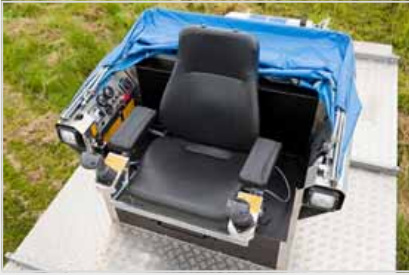
Ergonomic operator's seat with joysticks for operation/control of the machine and its tools.
